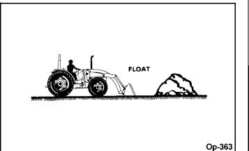
Float will also prevent mixing of surface material with stockpile material. Float position will reduce the chance of surface gouging when removing snow or other material.
